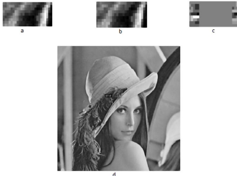
Fig.7. (a) the original block (b) the marked block with projection at angles (1,20) and (1,21) (c) the error block (d) the marked image
