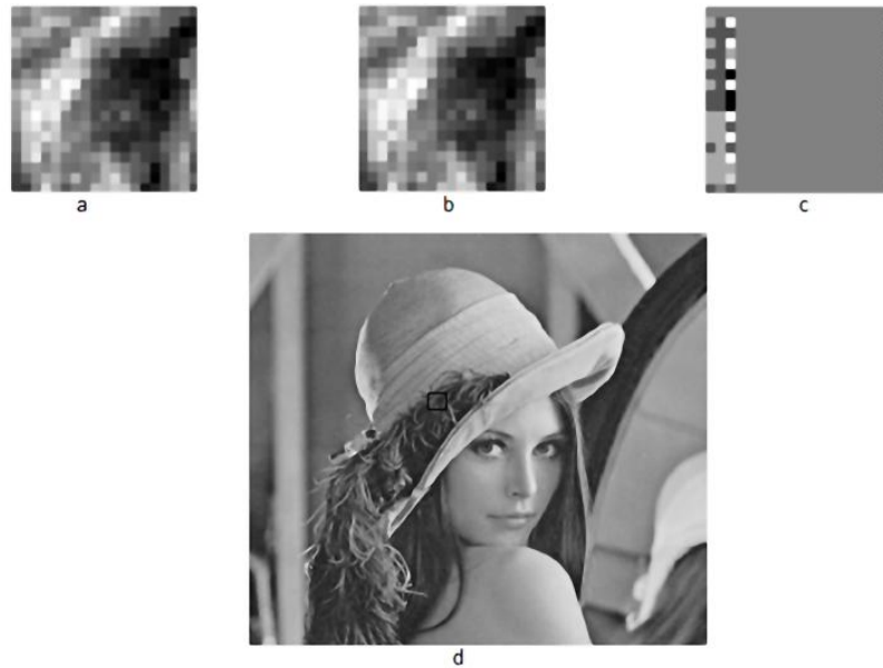
Fig.8. (a) the original block.(b) the marked block with projection at angles (1,16) and (1,18) (c) the error block (d) the marked image
