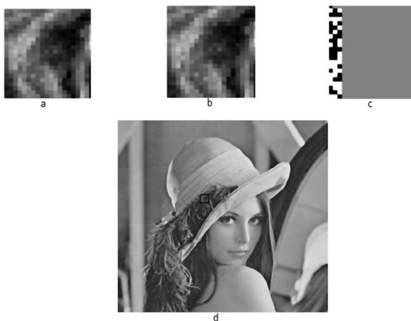
Fig.10. (a) the original block (b) the marked block with projection at angles (1,20) and (1,24) (c) the error block (d) the marked image
